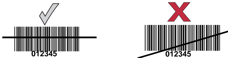
Figure 2-3 Acceptable and Incorrect Aiming
